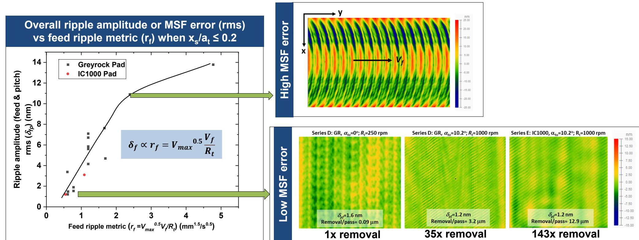
Combined feed & pitch ripple in a patch can be minimized when
