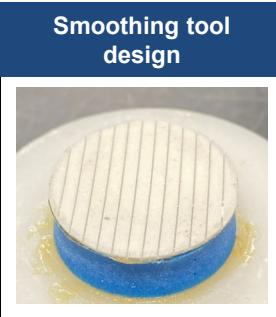
Reduces mid-spatial frequency (MSF) error w/o figure degradation
