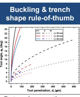
Determines optimum parameters ( $r_t, d_t, \alpha_{to}$ ) & trench cross section
