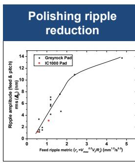
Determines process conditions to reduces MSF error
